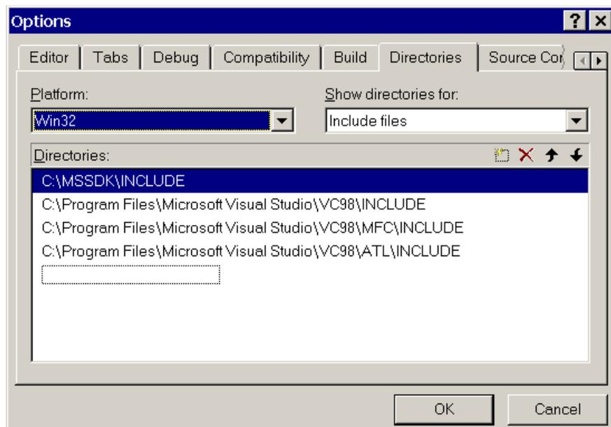
The topmost path indicates the folder that contains the latest DirectX header files. The default path is C:\Mssdk\Include. If the path is not present, add it to the list and move it to the top of the search list by using the toolbar controls within the **Directories** tab.
