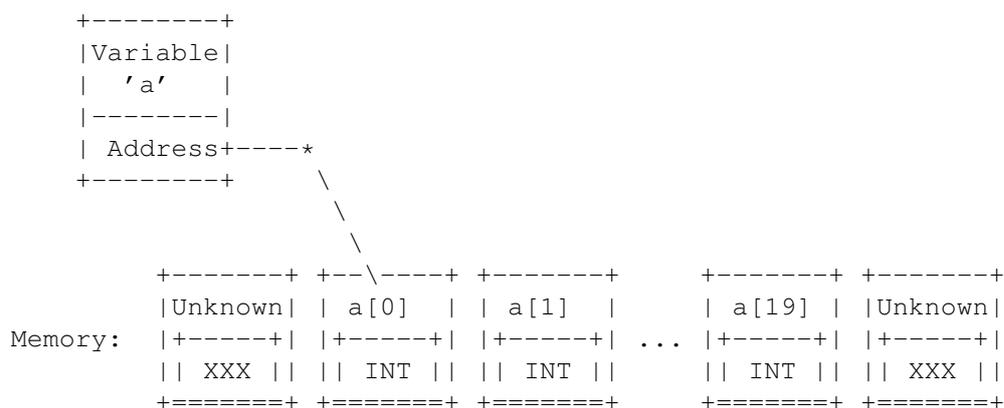
As you can see, the variable `a` is a pointer to the reserved chunk of memory which contains the array elements. Parts of memory that aren't between `a[0]` and `a[19]` are marked as 'Unknown' because they are not part of the array. This memory should therefore not be accessed using the array `a`.
