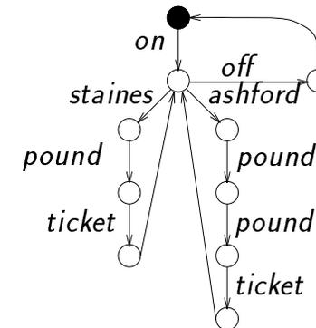
For any path through the diagram, starting from the black state, there is a trace consisting of the sequence of labels on the path.  $\text{traces}(\text{TICKETS})$  is the set of traces corresponding to all these paths, including  $\langle \rangle$  which corresponds to the empty path (i.e. simply remaining at the starting point).
