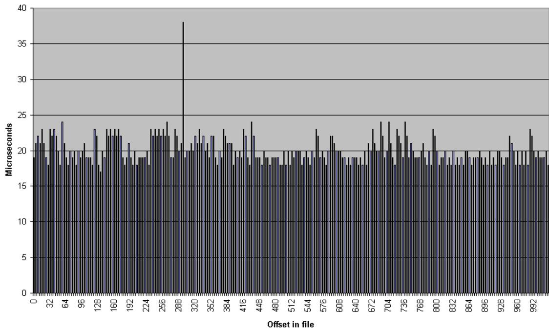
In the re-read latency graph one can clearly see the client side cache that is in NFS Version 3. The reread latencies are clearly not the latencies that one would get if the reads actually went to the NFS server and back.
