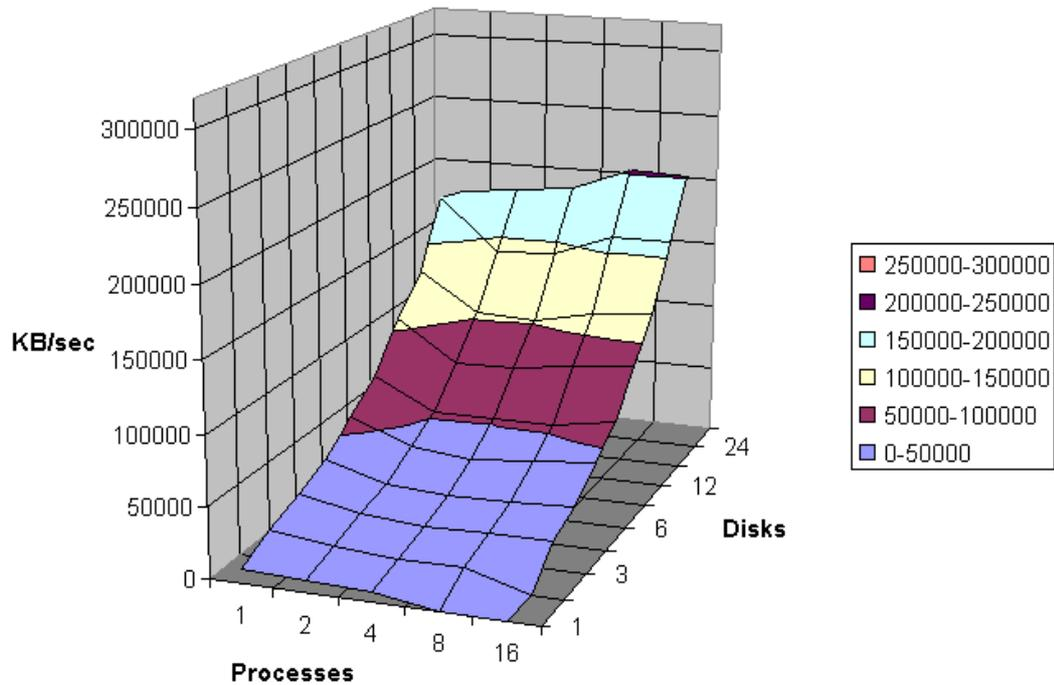
The graph above was created by running Iozone multiple times and then graphing the combination of the results. Here the graph is showing the throughput performance as a function of processes and number of disks participating in a filesystem. (disk striping) The good news is that on this system as one adds disks the throughput increases. Not all platforms scale so well.
