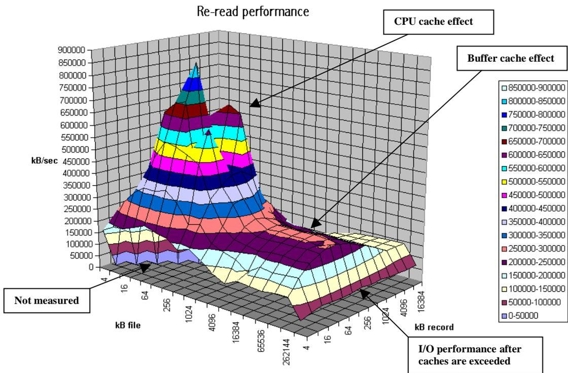
The graph above is displaying the impact of re-reading a file. Notice that the processor cache is now very important and causes the sharp peak. The next plateau to the right is buffer cache and finally above 256MB the file no longer fits in the buffer cache and real spindle speeds can be seen.
