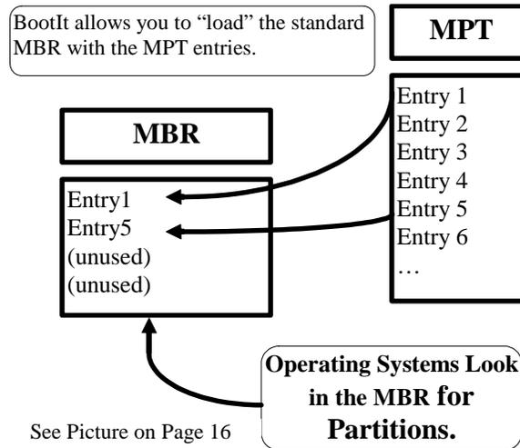
To get other partitions to show up in the operating system, as you can see from the figure above, you must assign the partitions to be loaded (up to four). Failure to correctly load the **MBR Details** section of the Boot Item—see the screen capture in *Set up the Normal Boot Menu* on page 16—is the most common cause of missing partitions.
