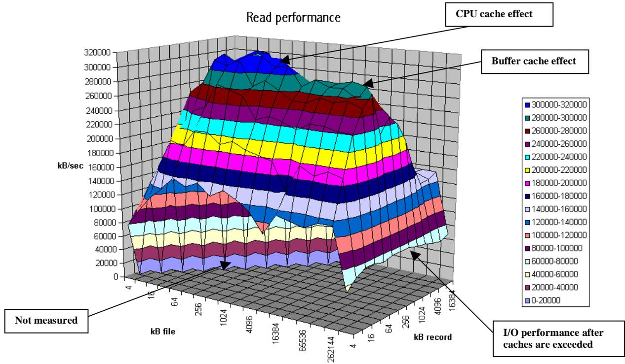
From the graph above one can clearly see the buffer cache helping out for file sizes that are less than 256MB but after that the actual disk I/O speed can be seen. Also note that the processor cache effects can be seen for file sizes of 16 Kbytes to 1Mbyte.
