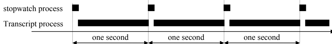
Figure 13.4. Higher priority stopwatch process taking turns with a lower priority process.
