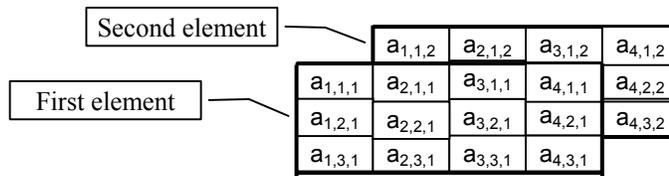
Figure 7.15. Three-dimensional array (three indices) as an array of two-dimensional arrays.
