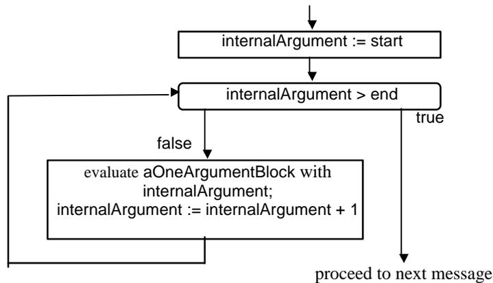
Figure 5.6. Execution of start to: end: do: aOneArgumentBlock.
