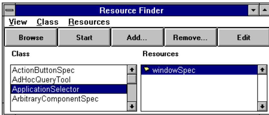
Figure 6.9. You can access an application with the Resource Finder. *Edit* opens the canvas editor, *Start* opens the application on the selected specification, *Browse* opens a browser on the application model class.
