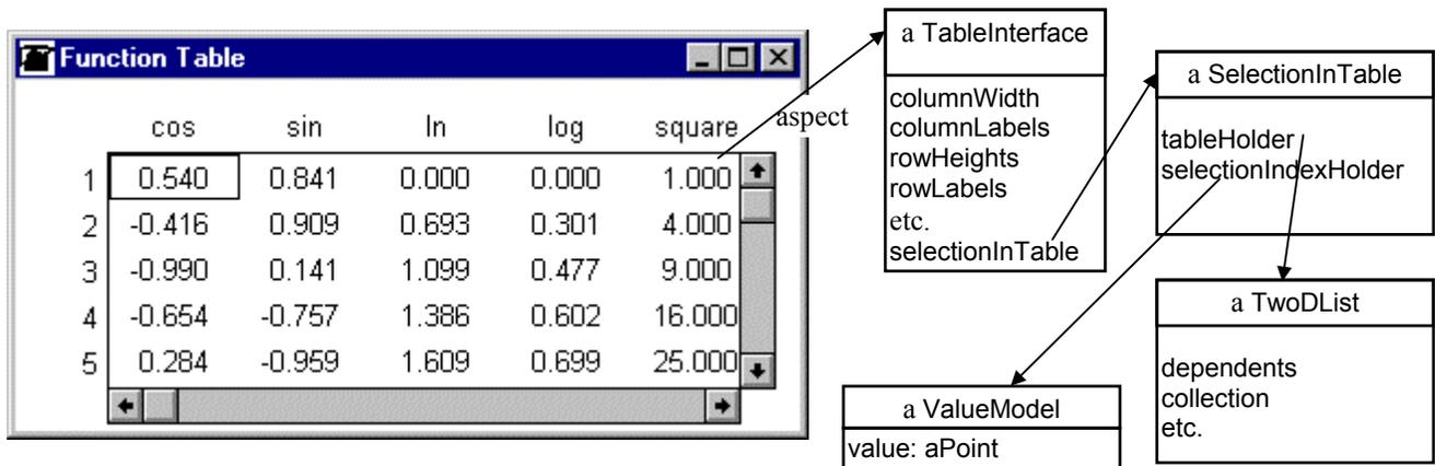
Figure 7.16. The structure of table widget support.
