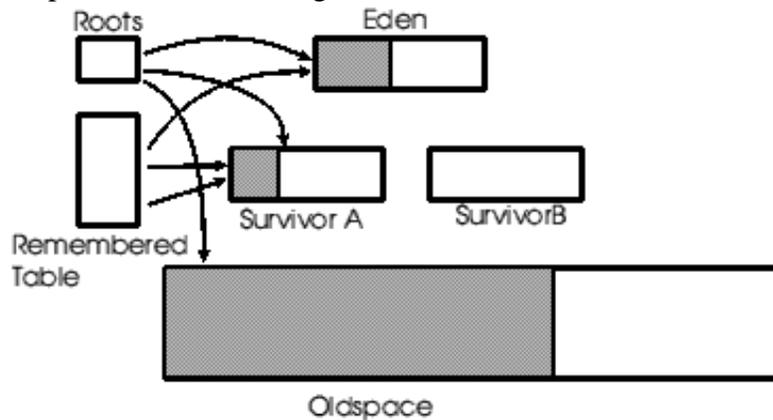
figure 8. Generation scavenging system before a scavenge
