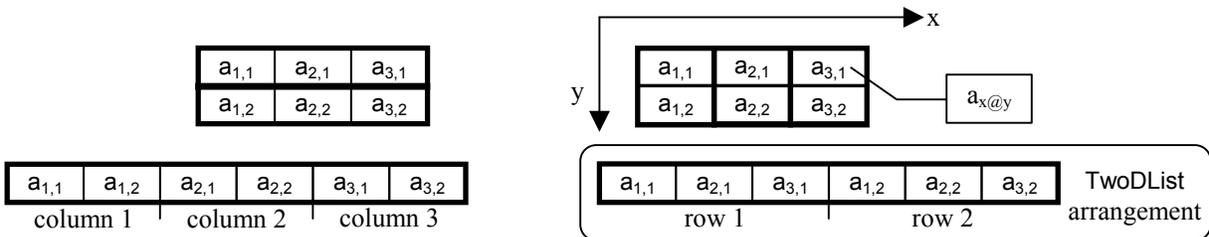
Figure 7.10. Tables can be stored as arrays of columns or rows (top) or as one-dimensional arrays (bottom). Class TwoDList uses the bottom right arrangement.
