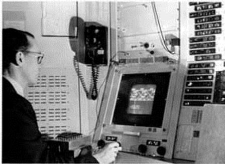
**Figure 1: Ivan Sutherland using Sketchpad (from <http://www.sun.com/960710/feature3/sketchpad.html>)**
