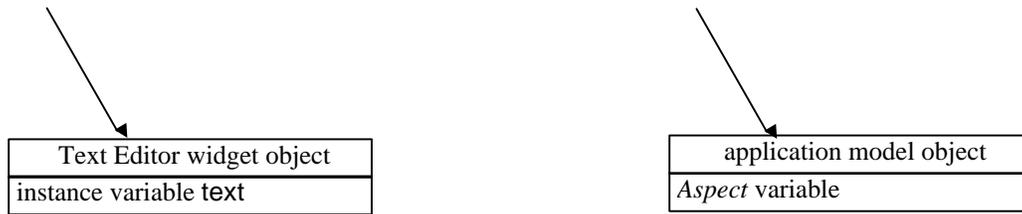
Figure 6.20. The text displayed in a Text Editor is stored in the widget's variable, the accepted text is stored in the *Aspect* variable in the application model.
